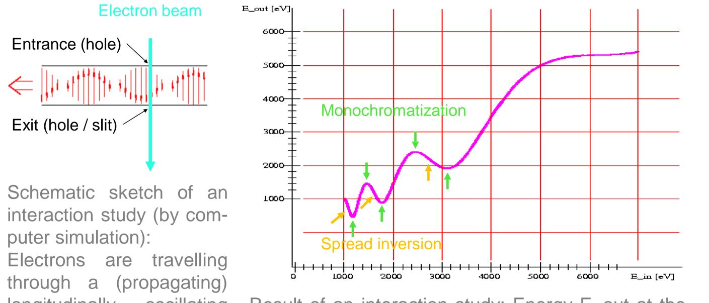
circular deflector links entrance time of electron with its azimuthal path position
